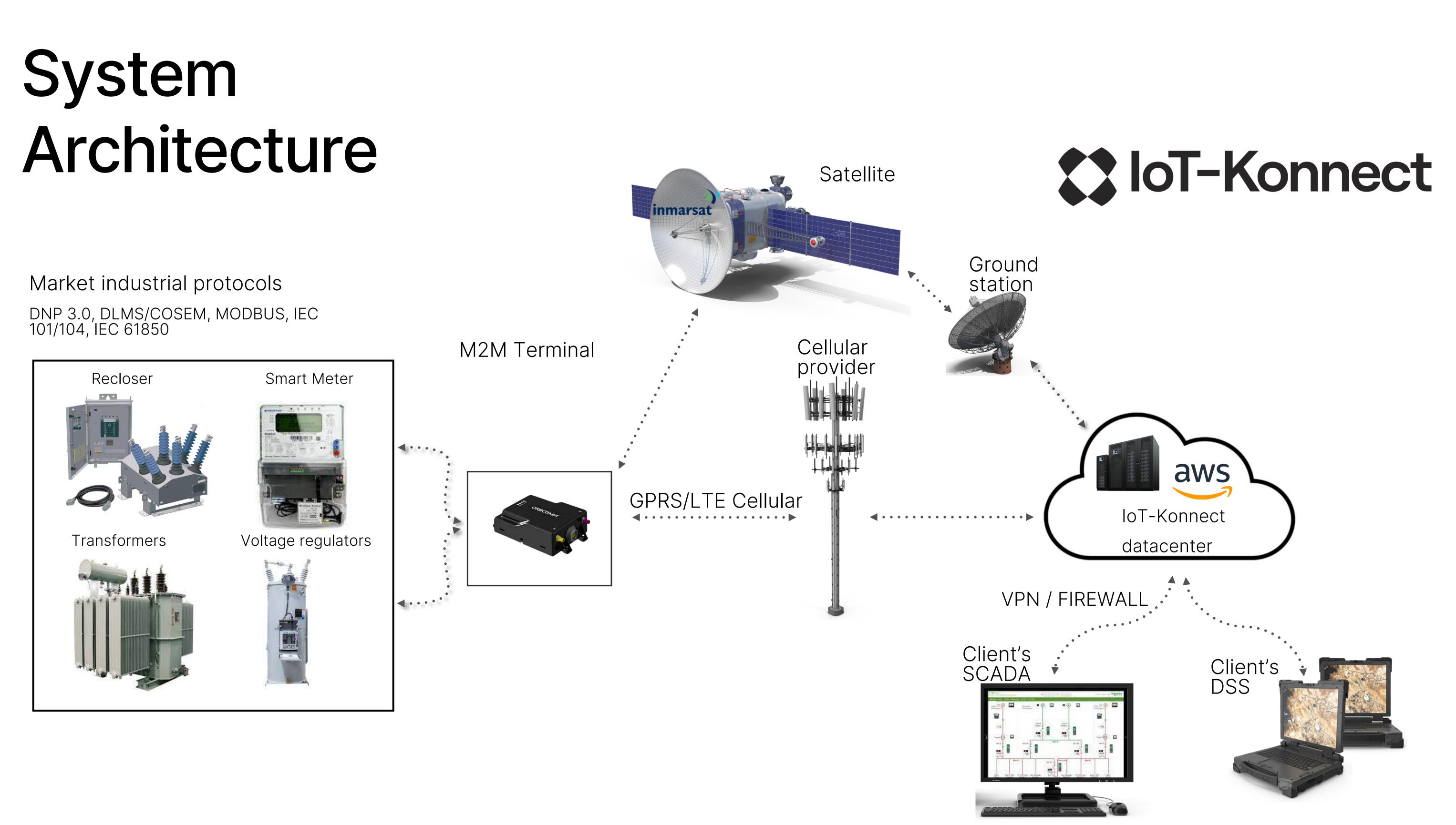
Our M2M terminal installed in the field is fully programmable and is in charge of communicate the slave device with your SCADA or DSS software. The signals are sent through a variety of communications options up to our middleware and then to your SCADA or DSS software, using encrypted and secure channels.
